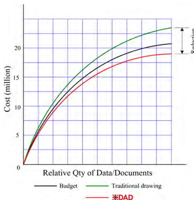
Fig. 11. Cost comparison between traditional CAD drawing and DAD.
