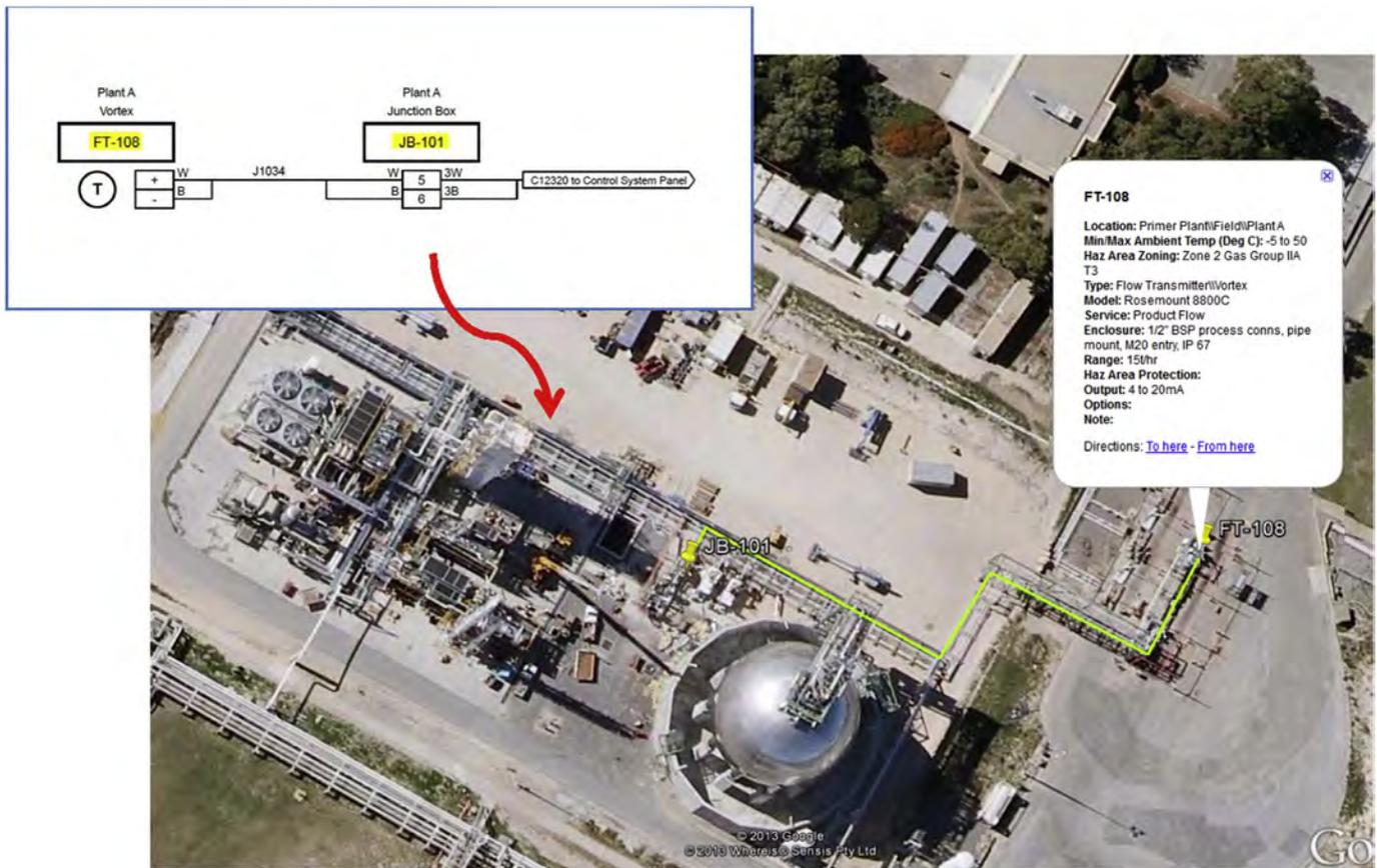
Fig. 13. Locating components with Google Map/Earth. (For interpretation of the references to colour in this figure, the reader is referred to the web version of this article.)
