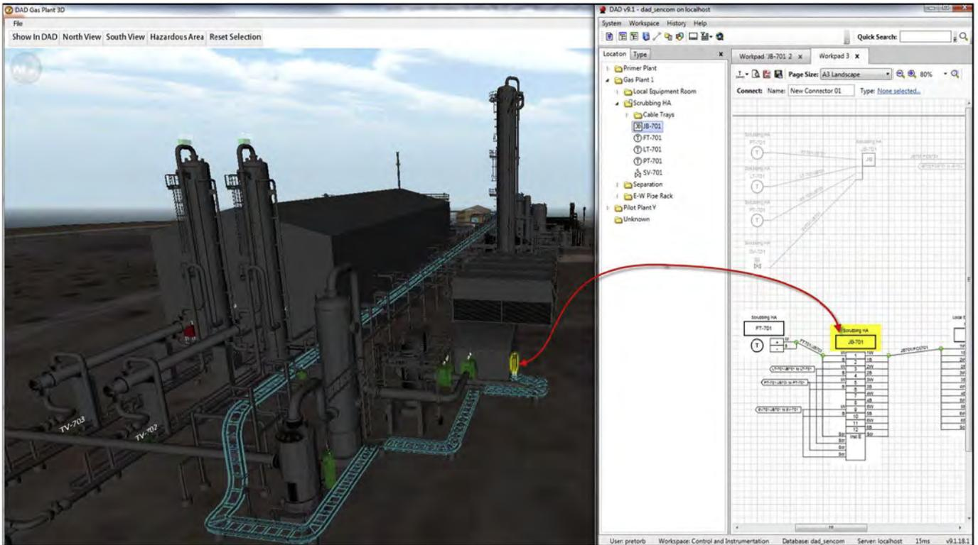
Fig. 15. Application in power plant construction. (For interpretation of the references to colour in this figure, the reader is referred to the web version of this article.)
